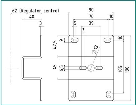
The mounting bracket set assures the secure mounting of the pressure regulators M59 und PR.
