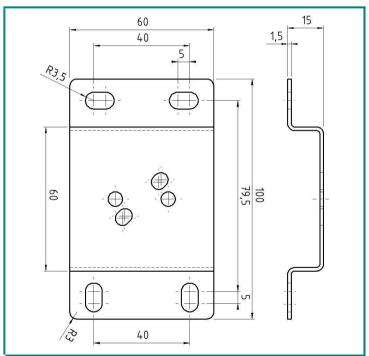
Wall mounting bracket in stainless steel and electrolytically polished and assures the secure mounting of the shut-off valve HP500 and the regulators HD400, HD250, HP300, HP310 and FR1.
