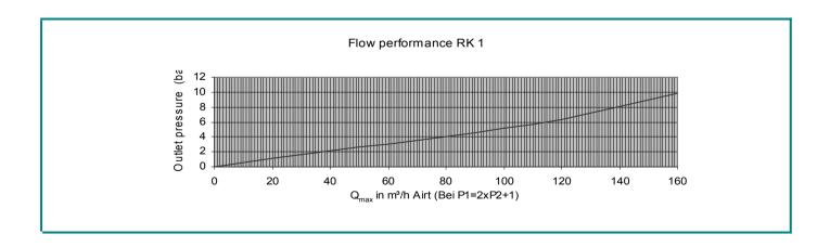
The pressure regulator RK 1 is for the installation in line systems with large gas flows. For example flame cutting installations. The RK 1 is in brass for flammable and non-flammable gases as well as stainless steel for corrosive gases.
