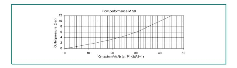
The cylinder regulator M 59 reduces the pressure of compressed gases as well as liquid gases from max.300 bar down to a max. pressure of 16 bar.
