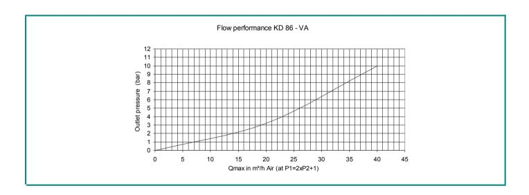
The KD 86 - VA is a regulator for corrosive gas and reduces, through two independent operating reduction stages, the max. cylinder pressure of 200 bar down to max. 16 bar.
