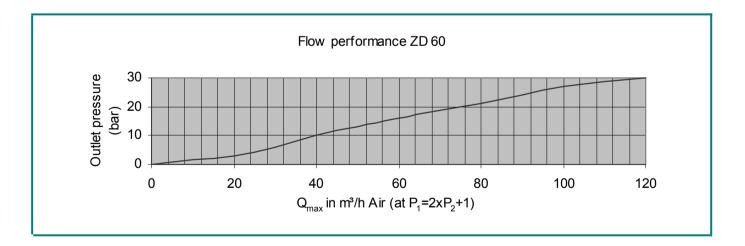
The central pressure regulator ZD 60 reduces a maximum inlet pressure from 300 bar down to 30 bar and kept constant. The ZD 60 is supplied in brass for non-corrosive, flammable (except acetylene) and non-flammable gases as well as stainless steel for corrosive gases.
