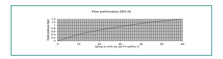
The supply station ZDA 25 is for the interruption free supply of Acetylene with manual switching from cylinder batteries and bundles. For 2x1 cylinder or max. 2x3 bundles. The supply station ZDA 25 consists of certified components: regulator, safety valve, quick connectors and check valve. Three-way ball valve for changing from empty to full batteries.
