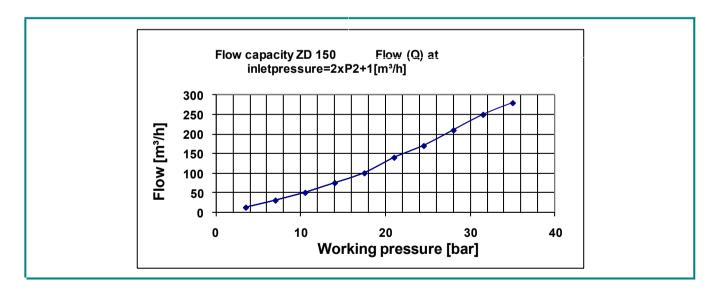
The central pressure regulator ZD 150 reduces a maximum inlet pressure from 300 bar down to 40 bar and kept constant. The ZD 150 is supplied in brass for non-corrosive, flammable (except acetylene) and non-flammable gases as well as stainless steel for corrosive gases.
